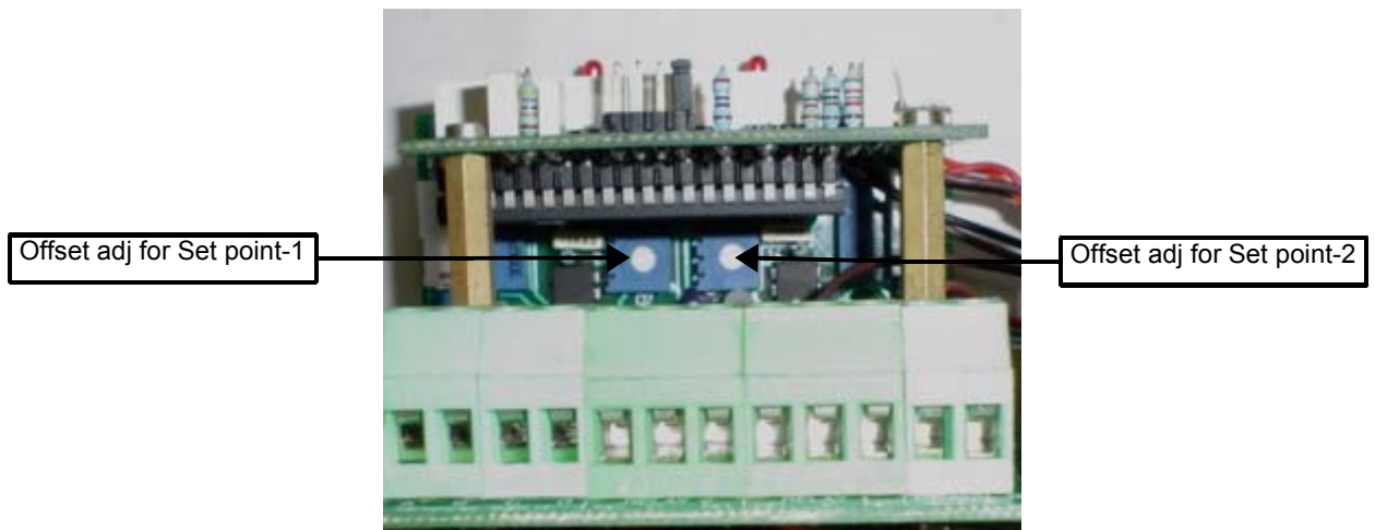
Fig-9: Alarm and control for Offset pot location
